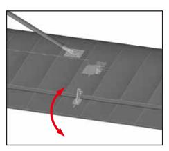
2A. To mount the undercarriage to the fuselage, start by inserting and securing the two rear braces with supplied 2x6mm screws (A). Now insert the main gear wire into the fuselage slot and slide the plastic brace keepers over the rear braces (B) to bring these two parts together. Insert the spring support wire between the main gear wire (C). Using supplied 6x4mm screws secure the main gear and spring support wire in place with the plastic undercarriage straps (D).
