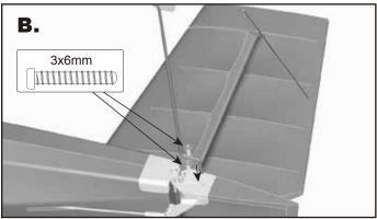
4. Insert one half of the carbon tail spar into one of the horizontal tail pieces before sliding this half into the tail slot on the fuselage. Now install the remaining tail piece (A). Secure both halves in place with the supplied 2.3x6mm screws and the elevator join with the single 2x8mm screw (B). This installation is self aligning, but do double check to ensure equal aliment to the vertical tail and wing.
