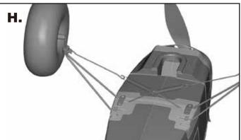
3. Insert the tail wheel assembly into the plastic slot on the bottom of the rudder and secure with two 3x6mm screws (A). The same method is used when mounting the water rudder (B)
