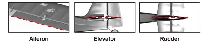
2. Check all control surfaces are moving in the correct direction with the correct stick input (see below).
