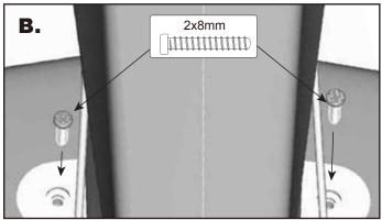
5. Using a pair of pliers (ball link pliers preferably) connect the elevator push rod to the elevator horn (A). To ensure both the elevator and rudder are neutral (with the servos centered) loosen the grub screw of the piano wire fastener and slide push rods until both surfaces are neutral if required (B). Tighten firmly when done. For added security, the tail can be glued in place too.
