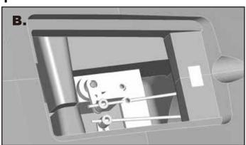
6. With the aileron control horns at 90 degrees to the wing surface (neutral) insert the aileron push rod and secure in place with plastic keepers (A). Connect the ball link to the aileron control horn as shown (B). Repeat this same process for the flaps, the exception being the flap servo horn must be positioned as far forwards as possible. This will give a flap neutral position with the push rod connected (C).
